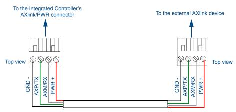
FIG. 5 Mini-Phoenix connector wiring diagram (direct data and power)
